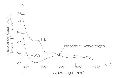
Figure 1. Optical absorption spectra of oxygenated  $(HbO_2)$  and de-oxygenated hemoglobin (Hb).
