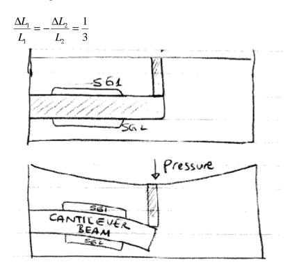
Gauge factor for both strain-gauges are given as:
