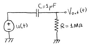
Where u(t) is a step function,  $R = 1 M\Omega$ ,  $C=1\mu F$  (fixed during the test)
