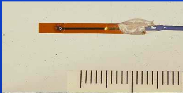
Single thin-film basis ion-selective electrode
