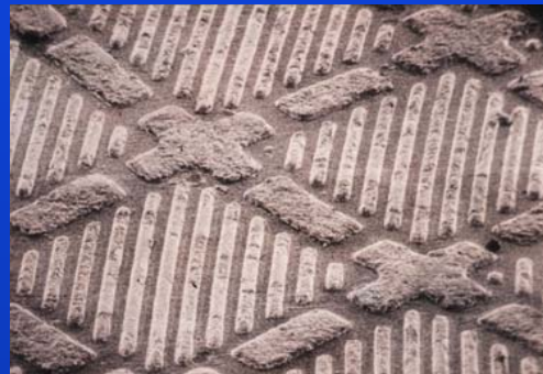
Micrograph of thick- film silicone dielectric strips
